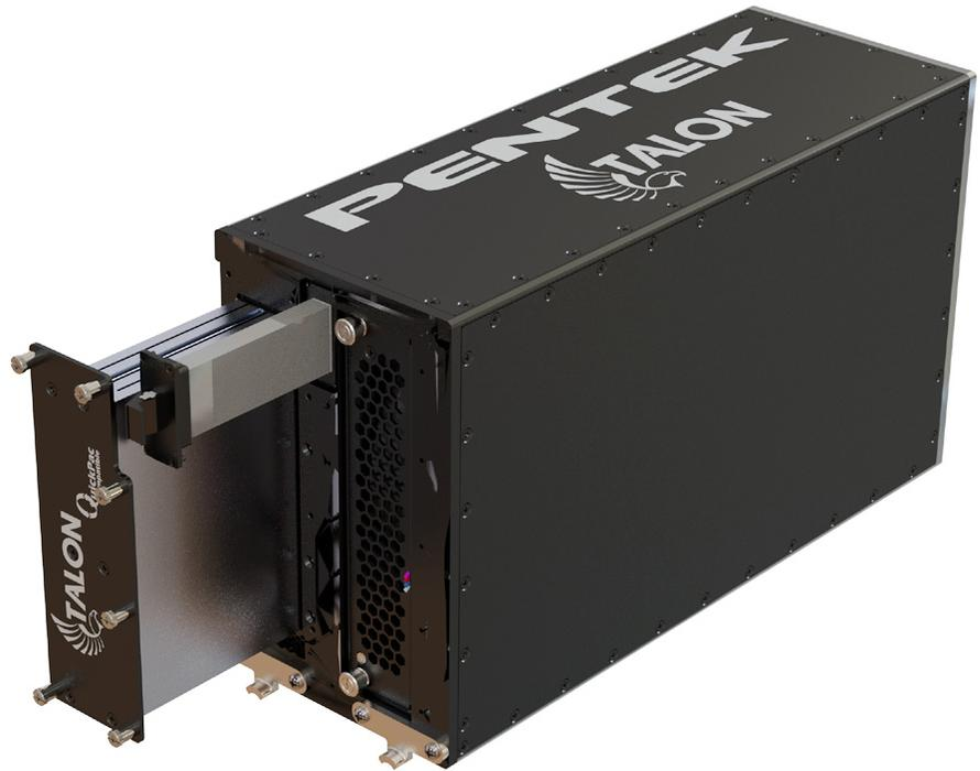
**Figure 2. Pentek's QuickPac™ drive pack provides up to 30 TB of solid state storage in a small package. These pictures show the QuickPac drive pack and OS drive removed and partially ejected from the Talon Model RTX 2589 3.6 GS/sec Ultra Wideband RF/IF Extreme 1/2 ATR Recorder.**
