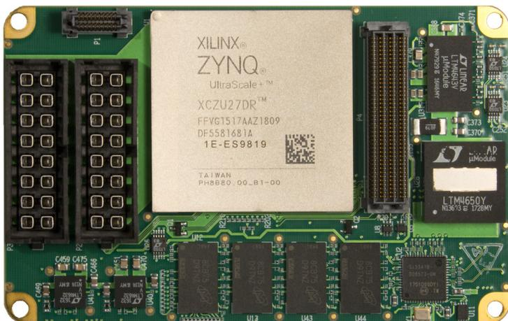
ual D/A outputs from the RFSoc are delivered to the carrier board through a multi-channel connector as differential pairs.
