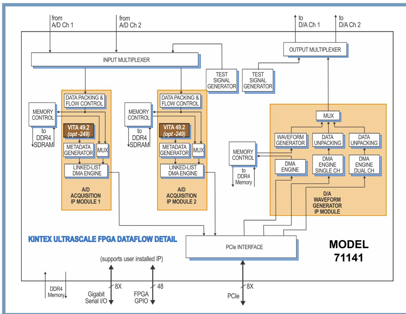
Precision time-stamping of the digitized elements is a key attribute of VITA 49.2. The Pentek IP automatically inserts timestamping information, per the VITA 49 standard, into the receiver stream data packets. The timestamp is applied at the A/D capture stage to generate the most accurate event capture time possible, regardless of data processing time.
