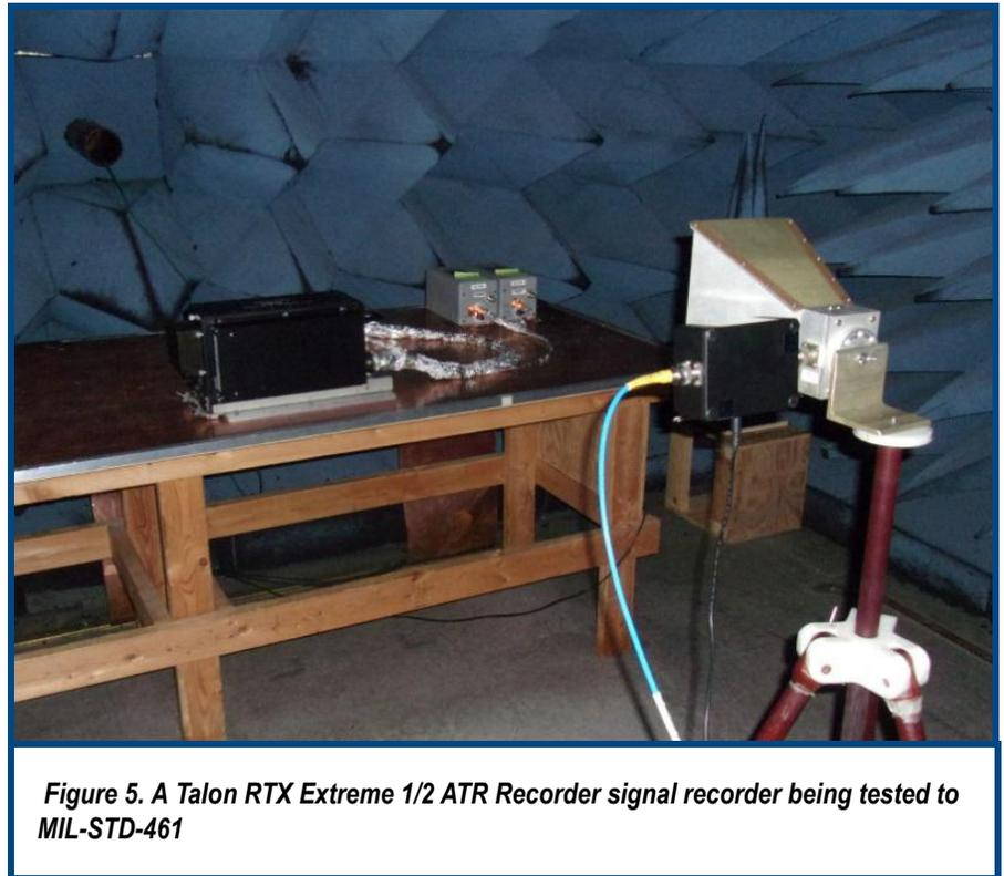
**Figure 5. A Talon RTX Extreme 1/2 ATR Recorder signal recorder being tested to MIL-STD-461**
