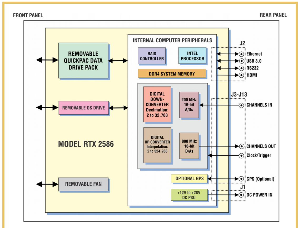
can replace a full one, minimizing mission down time. A companion offload system for the QuickPac drive pack is available so the recorder can remain in use while the recorded data is transported and reviewed via the offload system at a ground facility. The QuickPac drive pack holds up to 30.7 TB of solid state data storage capacity and supports RAID levels 0, 5, or 6.
