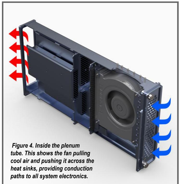
**Figure 4. Inside the plenum tube. This shows the fan pulling cool air and pushing it across the heat sinks, providing conduction paths to all system electronics.**
