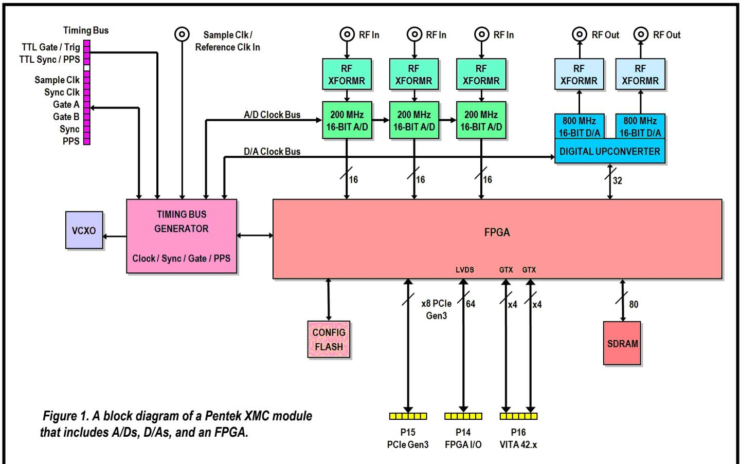
Figure 1. A block diagram of a Pentek XMC module that includes A/Ds, D/As, and an FPGA.
