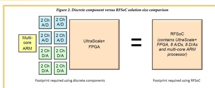
more exotic solutions like liquid and vapor cooling. RFSoC can easily bring power savings of 30% to 40% or more compared to typical discrete solutions, thereby reducing the cooling solution's complexity and weight. And in portable systems, every watt that can be eliminated results in smaller, lighter batteries and longer operation time.
