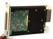
**3U VPX FlexorSet:** Fully integrated JadeFX carrier plus FMC module
