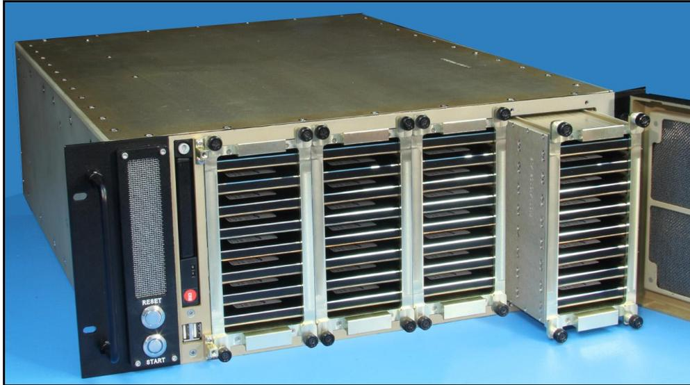
**Figure 2.** Pentek RTX 2766 ruggedized airborne recorder features four removable, hot swap QuickPac® drive packs, each containing eight SSDs in RAID arrays for easy transport of up to 60 TB of recordings to a secure facility.
