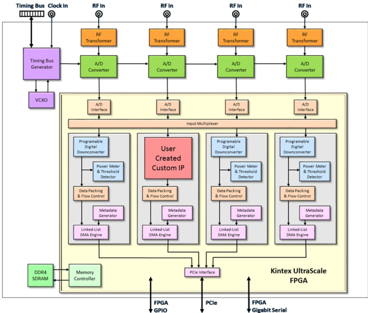
Figure 5. Jade Model 71861 Navigator FDK Design in IP Integrator
