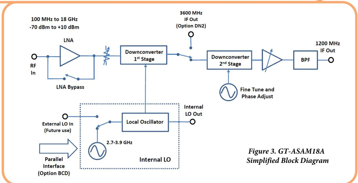
Figure 3. GT-ASAM18A Simplified Block Diagram
