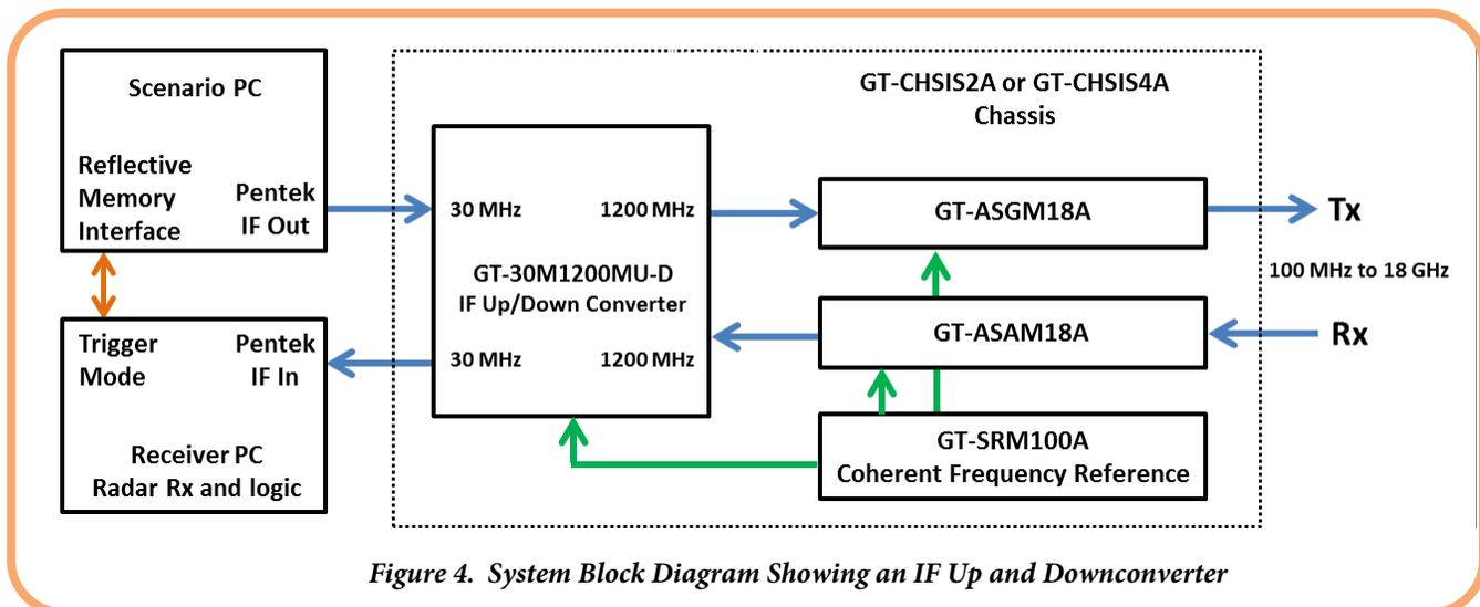
Figure 4. System Block Diagram Showing an IF Up and Downconverter
