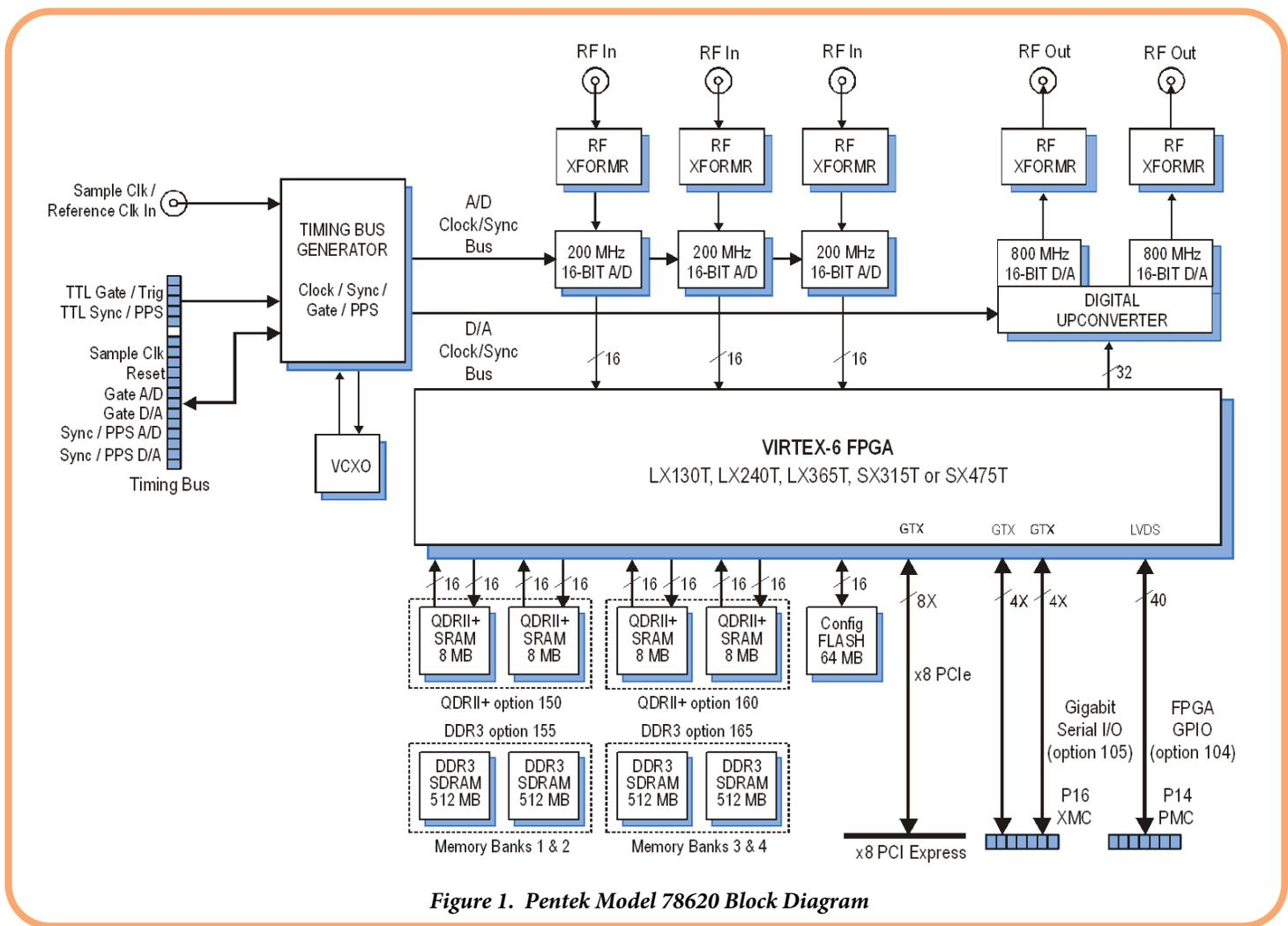
Figure 1. Pentek Model 78620 Block Diagram
