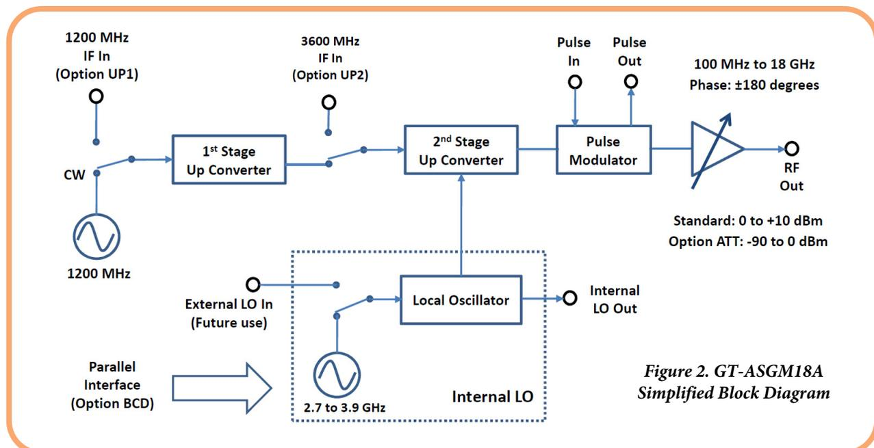
Figure 2. GT-ASGM18A Simplified Block Diagram
