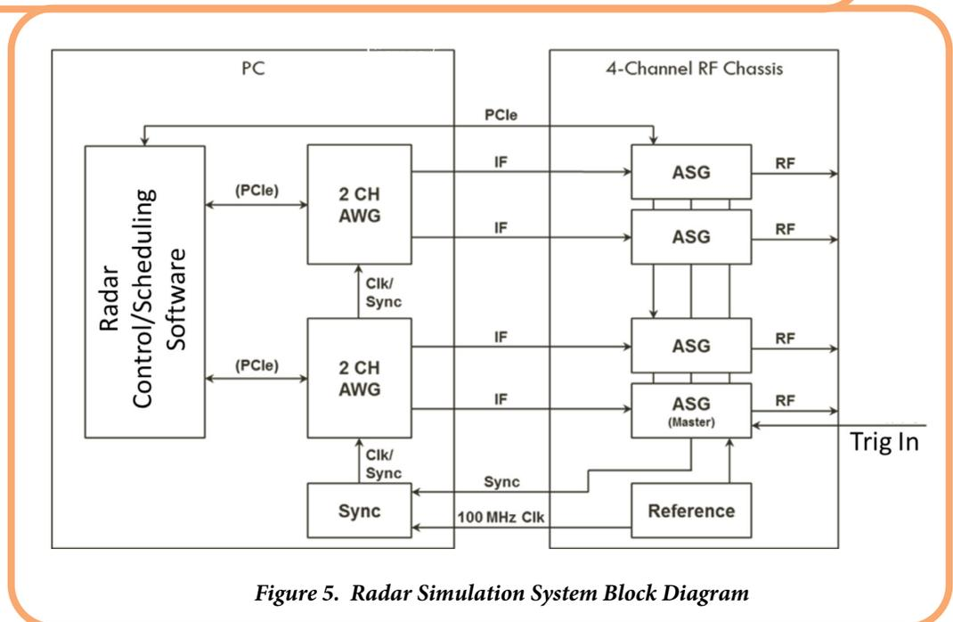
Figure 5. Radar Simulation System Block Diagram
