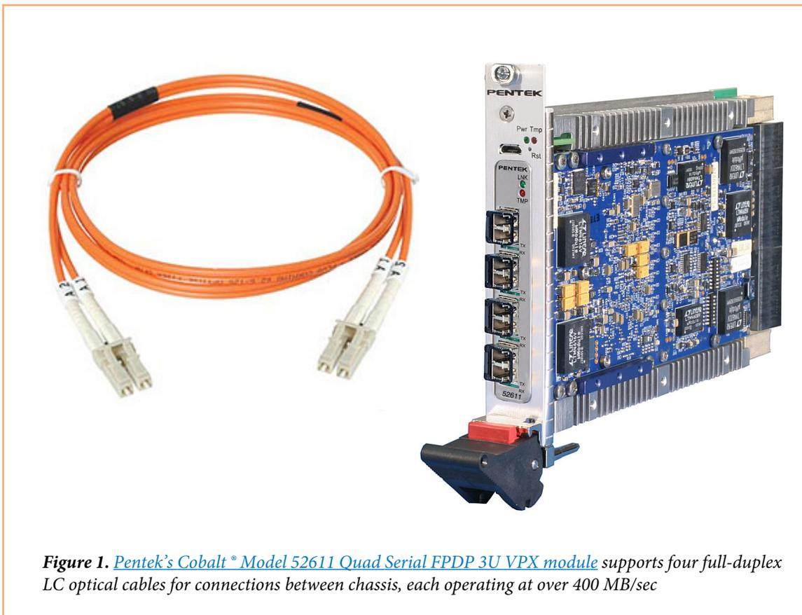
**Figure 1.** Pentek's Cobalt® Model 52611 Quad Serial FPDP 3U VPX module supports four full-duplex LC optical cables for connections between chassis, each operating at over 400 MB/sec
