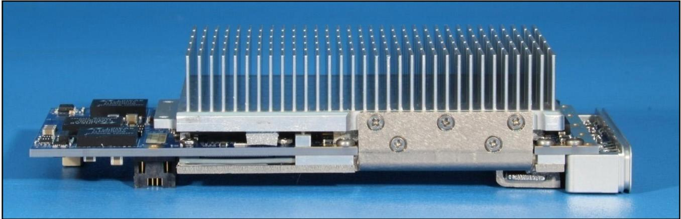
**Figure 3.** An air-cooled XMC module uses a highly-effective nickel-plated copper band to pull heat from a large FPGA on the underside of the board into an aluminum finned heat sink sitting in the airflow.
