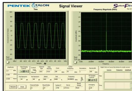
*Pentek's [SystemFlow Simulator](#) for Talon analog and digital recording systems includes a virtual recorder server application that simulates disk and I/O transactions for a complete and realistic recording environment.*
