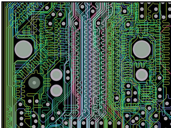
**Figure 1.** Length matching between circuit board traces of gigabit serial links requires extra loops and curves to ensure simultaneous arrival at the receivers.
