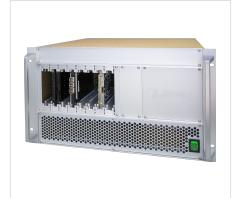
The 8256 is a SOSA aligned 3U VPX chassis ideal for application development with Mercury's RFSoC based Quartz<sup>®</sup> data acquisition and processing boards. Working
