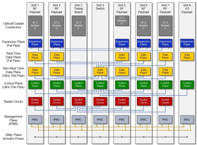
\_\_\_\_\_ Note: Expansion Plane interfaces are not wired on backplane, but can be connected using the Meritec Cabling System
