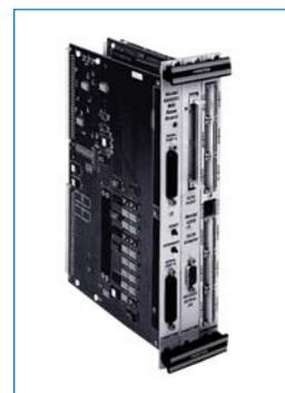
*16-channel data acquisition and signal analysis system fits in just three VMEbus slots. System consists of a 4270, a 4255 SCSI Interface MIX module, a 4252 16-channel 16-bit A/D and D/A Converter MIX module, all stacked on a 4200A MIX Baseboard.*
