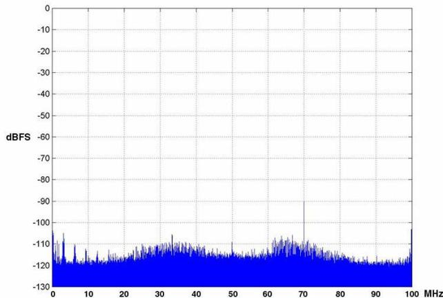
$f_{in} = 70 \text{ MHz}$ ,  $A_{in} = 0 \text{ dBFS}$ ,  $f_s = 200 \text{ MHz}$ , Int. Clock
