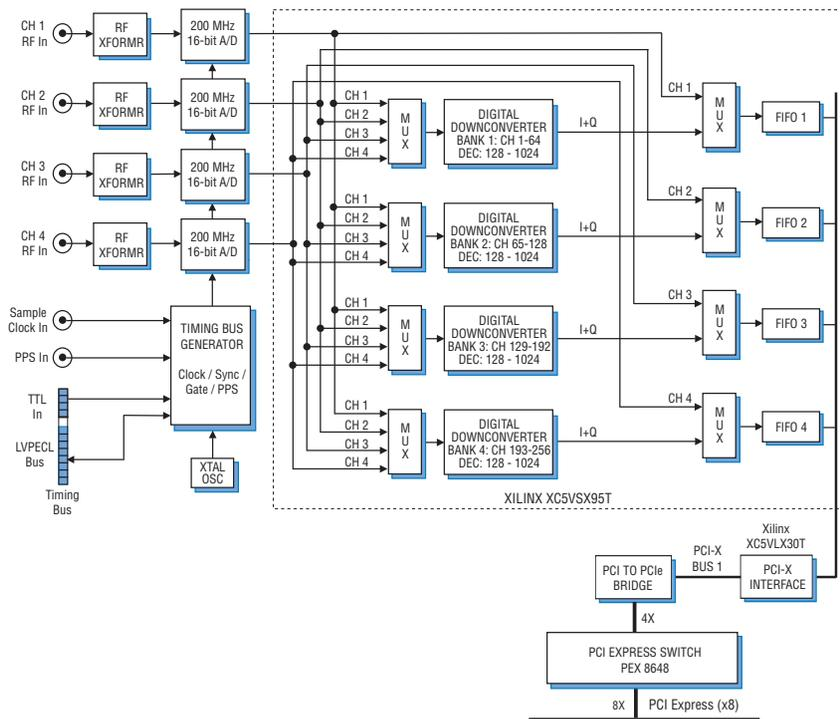
► Each of the output FIFOs operates at its own input and output rate to support different DDC decimation settings between the banks and efficient block transfers to the PCI bus.
