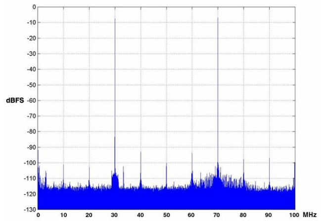
$f_{in1} = 30 \text{ MHz}$ ,  $f_{in2} = 70 \text{ MHz}$ ,  $f_s = 200 \text{ MHz}$ , Int. Clock
