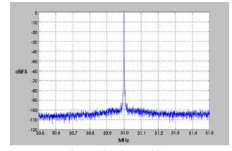
${\rm f_{in}} = 69~{\rm MHz}, \, {\rm f_s} = 100~{\rm MHz}$  Phase Noise @ 100 kHz = -102 - 10\*log(610) = -129.8 dB/Hz
