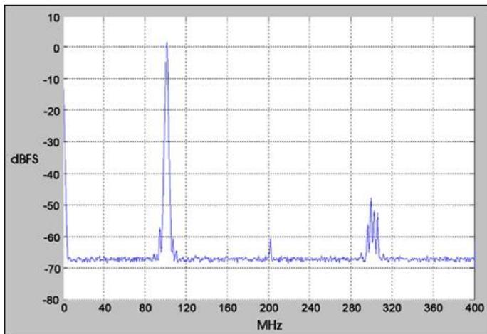
$f_{out} = 100$  MHz,  $f_s = 800$  MHz, Interpolation = 4,
