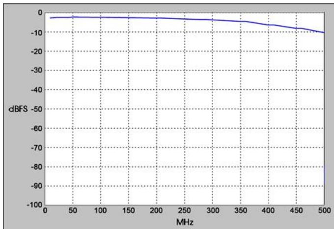
$f_s = 200 \text{ MHz}, \text{Internal Clock}$
