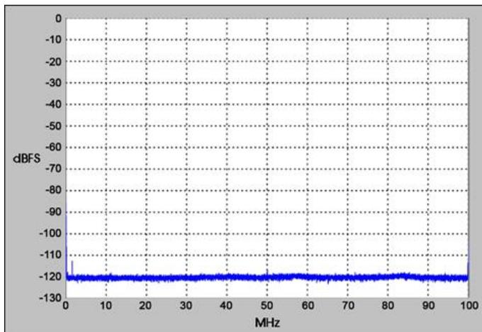
$f_s = 200 \text{ MHz}, \text{Internal Clock}$
