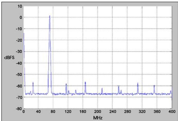
$f_{out} = 70$  MHz,  $f_s = 800$  MHz, Interpolation = 4,
