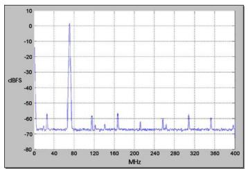
$f_{out} = 70 \text{ MHz}, f_s = 800 \text{ MHz}, Interpolation} = 4,$  Internal Clock
