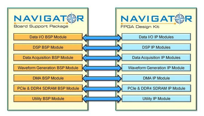
Because all Pentek boards are shipped with a full suite of built-in IP functions and numerous software examples, new applications can be developed by building on the provided software examples or built entirely new with the BSP extensive libraries. All BSP libraries are provided as C-language source for full access and code transparency.
