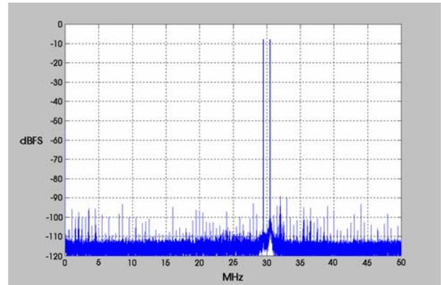
$f_1 = 29.5 \text{ MHz}, f_2 = 30.5 \text{ MHz}, f_s = 100 \text{ MHz}$
