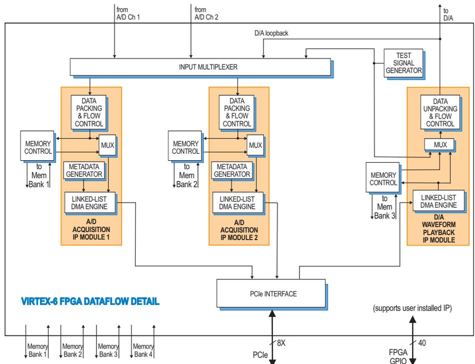
► module's DMA capabilities, providing FIFO memory space for creating DMA packets. For applications requiring deep memory resources, DDR3 SDRAM banks can each be up to 512 MB deep. Built-in memory functions include an A/D data transient capture mode and D/A waveform playback mode.
