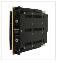
The 5586 is a high-performance, SOSA aligned 3U OpenVPX coprocessor board based on the Xilinx Virtex UltraScale+ HBM FPGA.
