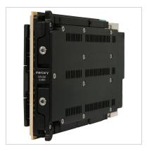
The 5585 SOSA aligned 3U OpenVPX board is an 8-channel, highspeed data converter with programmable DDCs (digital downconverters). It is suitable for connection to HF or IF ports of a communications or radar system. Its built-in data capture feature offers an ideal turnkey solution as well as a platform for developing and deploying custom FPGA-processing IP.
