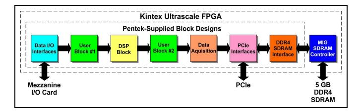
Along with the Navigator FDK, ArchiTek provides the foundation and example projects for adding IP to user blocks and creating additional data path branches from an existing data streams. The structured design protects custom IP developers from breaking the recorder's standard functionality, reducing development time and risk.
