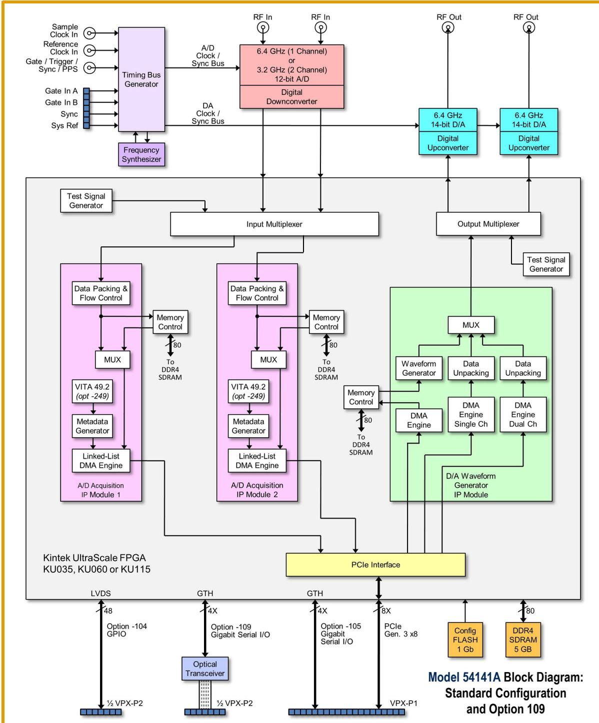
with an equally impressive reductions in cost, power dissipation, and weight. As the central feature of the Jade Architecture, the FPGA has access to all data and control paths, enabling factory-installed functions including data multiplexing, channel selection, data packing, gating, triggering and memory control. A 5 GB bank of
