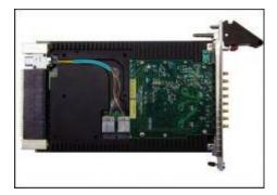
Pentek Model 5973 3U OpenVPX FMC carrier with VITA 66.4 optical backplane interface supports 12 GBytes/sec of traffic in and out of the module over 24 optical fibre lanes to a remote SFF subsystem.
