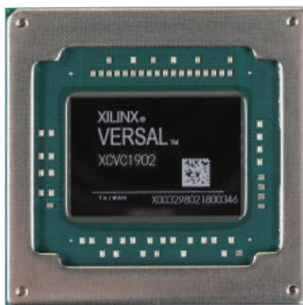
The VERSAL adaptive compute acceleration platform (ACAP) from Xilinx represents a new category of heterogeneous compute devices that the company says features "capabilities that far exceed those of conventional CPUs, GPUs, and FPGAs."
