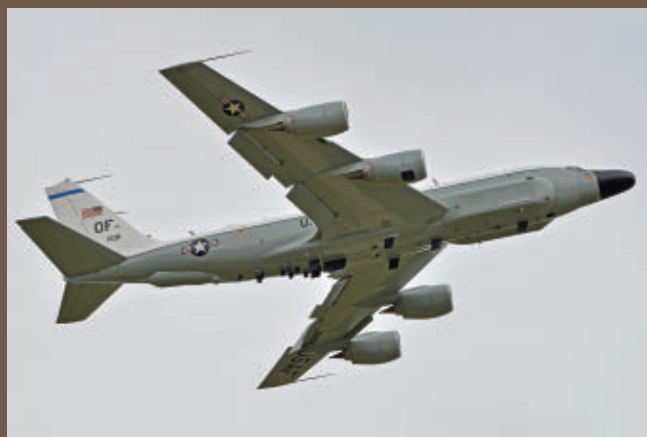
This US Air Force RC-135W Rivet Joint, seen taking off from RAF Mildenhall in the UK, displays a variety of SIGINT antennas, such as the blade antennas beneath the fuselage, as well as “cheek” arrays behind the cockpit.
