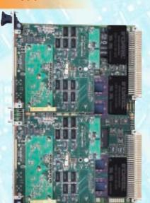
Model 4294 shown with two VIM modules installed
