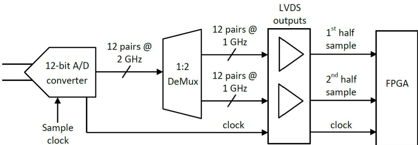
Figure 6. Parallel versus serial PCB routing
