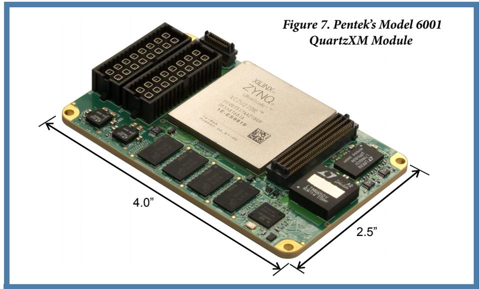
**Figure 7. Pentek's Model 6001 QuartzXM Module**
