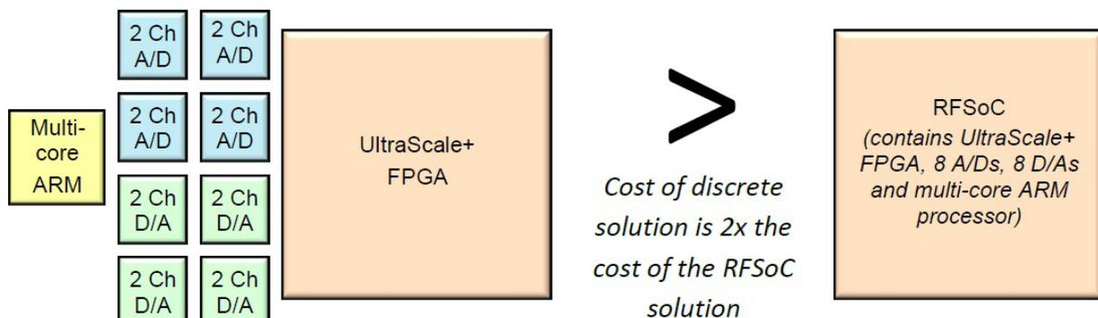
A/D and D/A pair combined with signal generation and receive and control processing. With these systems as well as military surveillance and targeting systems where hundreds of elements can be required, the savings found in RFSoc's integrated solution can add up quickly.
