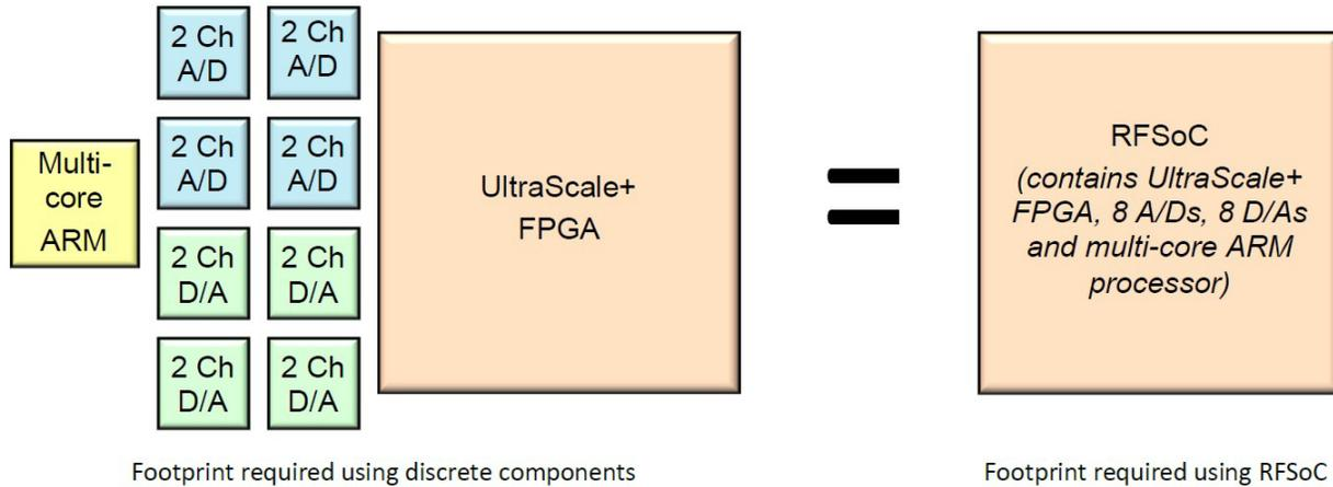
more exotic solutions like liquid and vapor cooling. RFSoc can easily bring power savings of 30% to 40% or more compared to typical discrete solutions, thereby reducing the cooling solution's complexity and weight. And in portable systems, every watt that can be eliminated results in smaller, lighter batteries and longer operation time.
