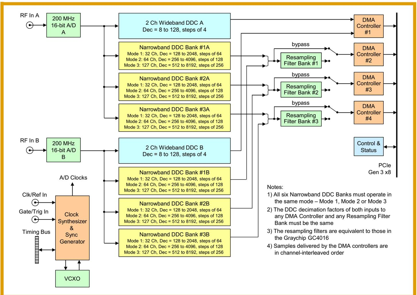
delivered to four DMA controllers linked to the PCIe Gen.3 x8 interface for transfer to a signal processor.
