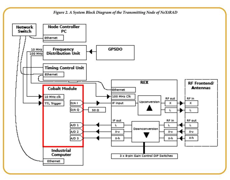
resolution of three meters. Each node has dual-polarized L- and X-band antennas (IEEE definition) with a 10-degree beamwidth.
