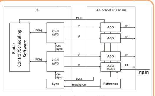
Figure 5. Radar Simulation System Block Diagram
