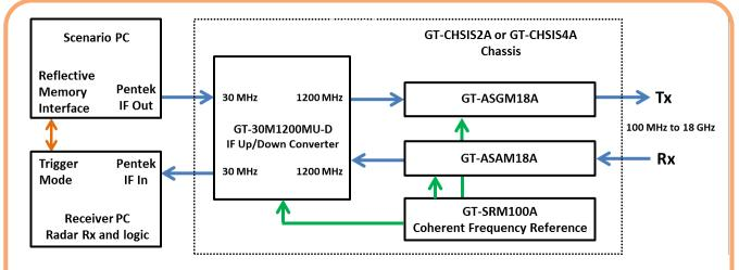
Figure 4. System Block Diagram Showing an IF Up and Downconverter
