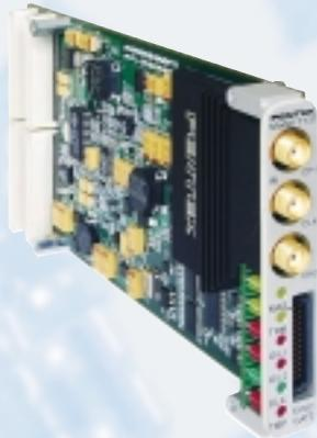
*Model 7131 is a 16-channel multiband digital receiver PMC module, that includes 14-bit A/Ds and a Virtex-II FPGA.*
