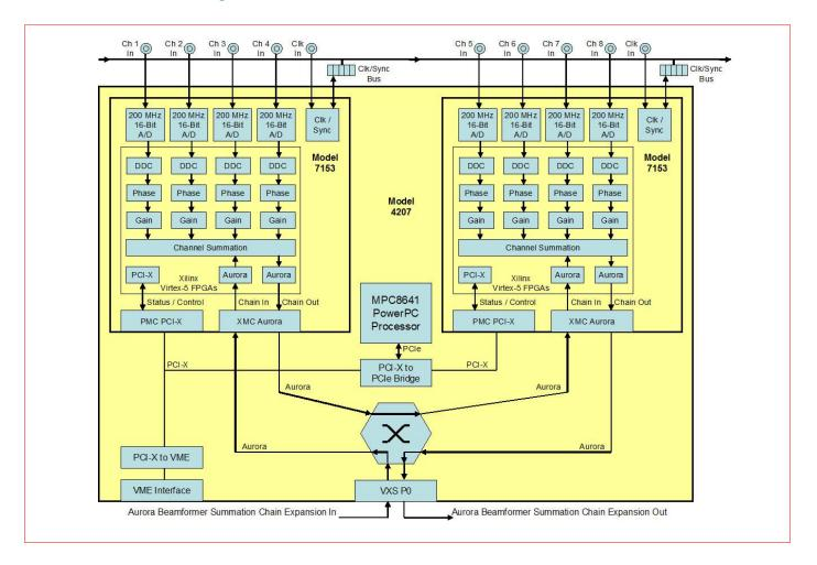
The Model 7153 PMC module is high-speed digitizer featuring four 200 MHz 16-bit A/Ds with a high-performance 4-Channel DDC. Two such modules mounted on the Model 4207 PowerPC I/O processor can be used to create an 8-channel beamforming system. Two or more of these systems can be joined together to create multichannel systems with higher density.
