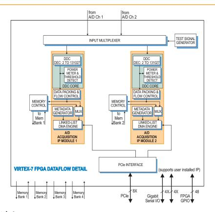
➤ In this case the IF signal frequency is chosen by setting an appropriate VCO tuning frequency, A/D sample clock frequency, and DDC decimation factor to achieve optimal flatness, anti-aliasing, SNR and SFDR performance, based on the Maxim 2121 datasheet specifications. All three of these parameters are programmable by the user
