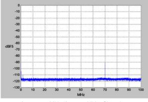
$f_{in Ch2} = 70 \text{ MHz}, f_s = 200 \text{ MHz}, Ch 1 \text{ shown}$
