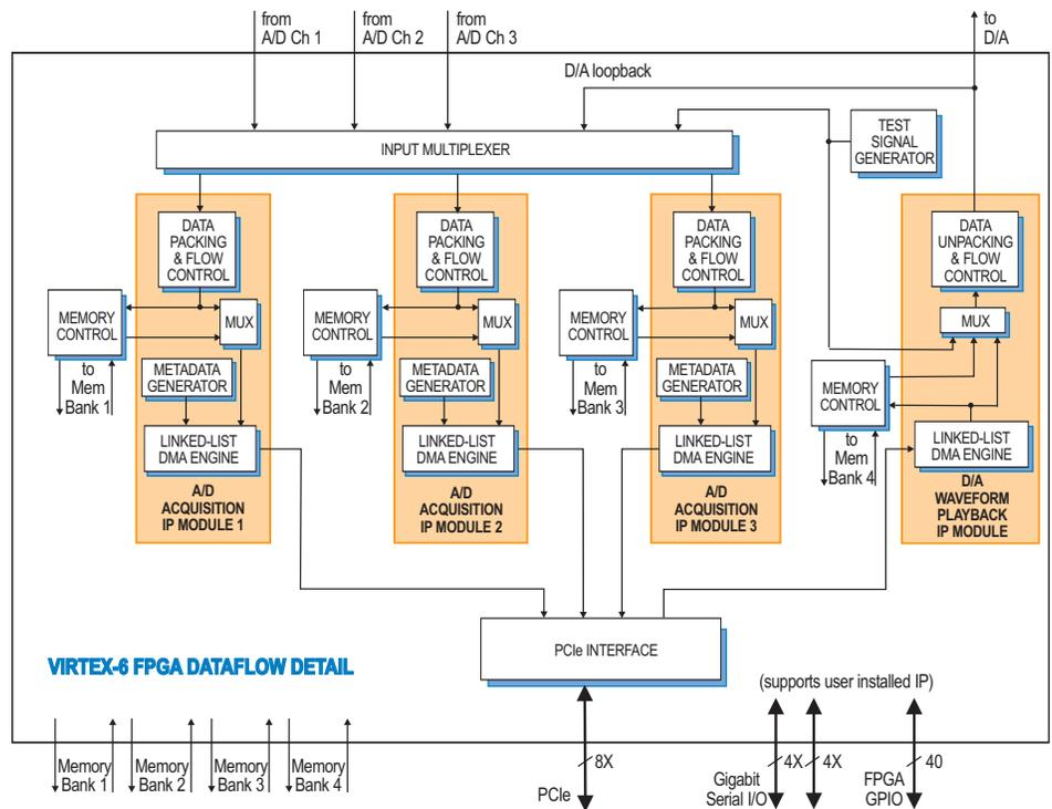
► board's DMA capabilities, providing FIFO memory space for creating DMA packets. For applications requiring deep memory resources, DDR3 SDRAM banks can each be up to 512 MB deep. Built-in memory functions include an A/D data transient capture mode and D/A waveform playback mode.
