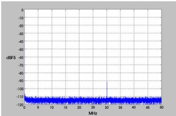
$f_{in \text{ Ch2}} = 69 \text{ MHz}, f_s = 100 \text{ MHz}, \text{ Ch 1 shown}$
