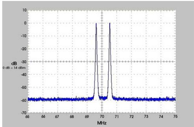
$f_1 = 69.5 \text{ MHz}$ ,  $f_2 = 70.5 \text{ MHz}$ ,  $f_s = 100 \text{ MHz}$
