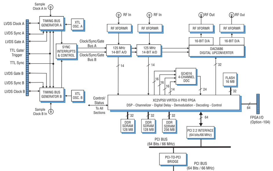
► the timing source for the A/Ds, the down-converter, the upconverter and the D/As. Two external reference clocks are accepted, one for each timing bus and two internal clocks may be used for each timing bus.
