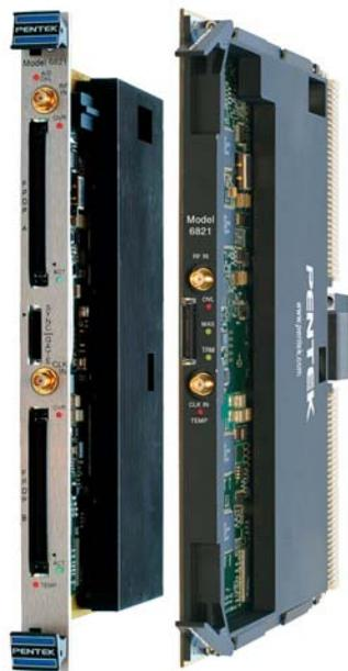
Model 6821-422 commercial (left) and conduction-cooled version.
