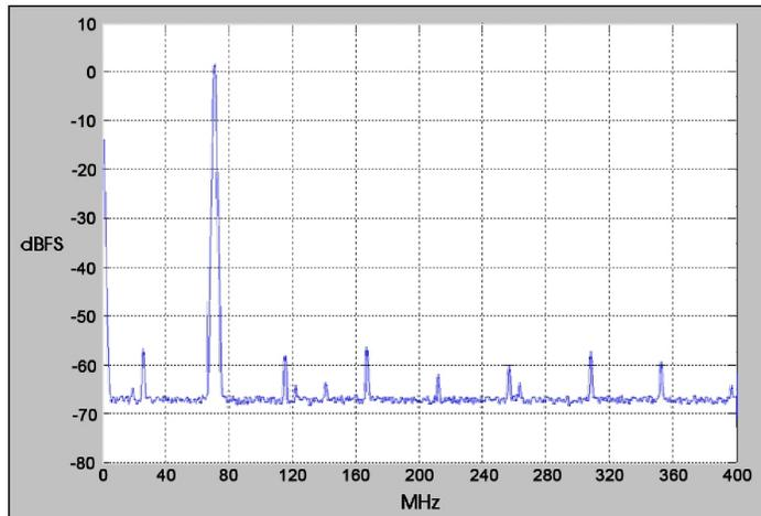
$f_{out} = 70 \text{ MHz}$ ,  $f_s = 800 \text{ MHz}$ , Interpolation = 4,
