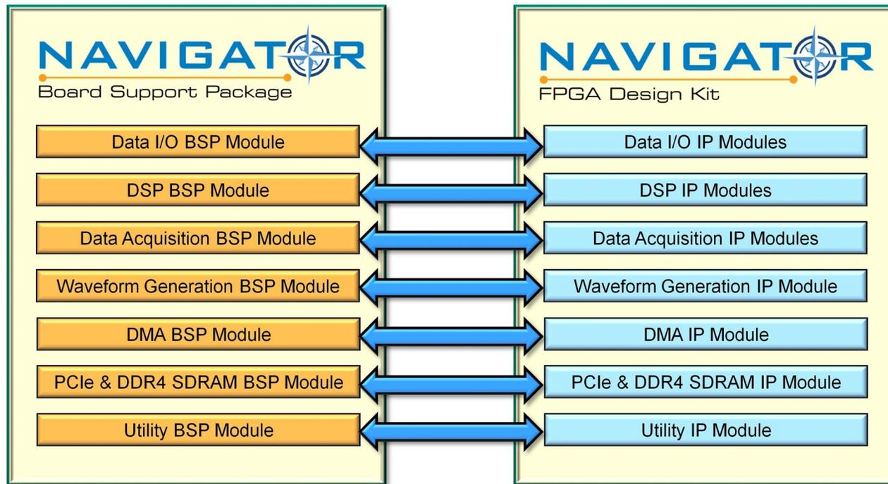
Because all Pentek boards are shipped with a full suite of built-in IP functions and numerous software examples, new applications can be developed by building on the provided software examples or built entirely new with the BSP extensive libraries. All BSP libraries are provided as C-language source for full access and code transparency.
