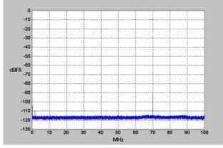
$f_{in Ch2} = 70 MHz$ ,  $f_{s} = 200 MHz$ , Ch 1 shown
