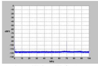
$f_{in Ch2} = 70 \text{ MHz}, f_{s} = 200 \text{ MHz}, Ch 1 \text{ shown}$
