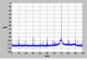
$f_{in} = 70$  MHz,  $f_s = 200$  MHz, Internal Clock
