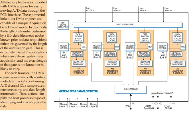
acquisition and the exact length of that gate is not known or is likely to vary. For each transfer, the DMA engine can automatically construct metadata packets containing A/D channel ID, a sample-accurate time stamp and data length information. These actions simplify the host processor's job of
