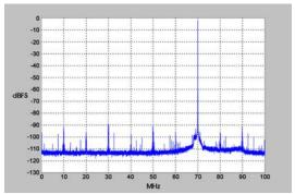
$f_{in} = 70$  MHz,  $f_{s} = 200$  MHz, Internal Clock
