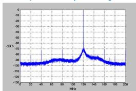
$\rm f_{out}$  = 140 MHz,  $\rm f_{s}$  = 400 MHz, External Clock
