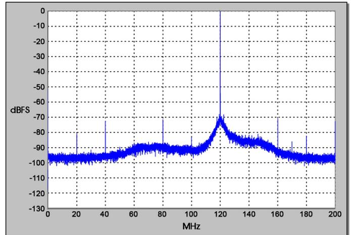
$f_{\text{out}} = 120 \text{ MHz}$ ,  $f_{\text{s}} = 400 \text{ MHz}$ , External Clock
