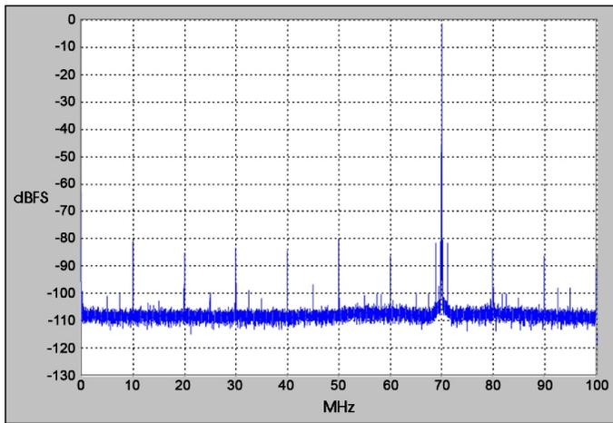
$f_{\text{out}} = 70 \text{ MHz}$ ,  $f_{\text{s}} = 200 \text{ MHz}$ , Internal Clock
