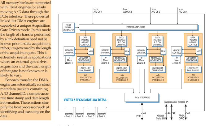
likely to vary. For each transfer, the DMA engine can automatically construct metadata packets containing A/D channel ID, a sample-accurate time stamp and data length information. These actions simplify the host processor's job of identifying and executing on the data.
