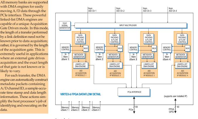
For each transfer, the DMA engine can automatically construct metadata packets containing A/D channel ID, a sample-accurate time stamp and data length information. These actions simplify the host processor's job of identifying and executing on the data.
