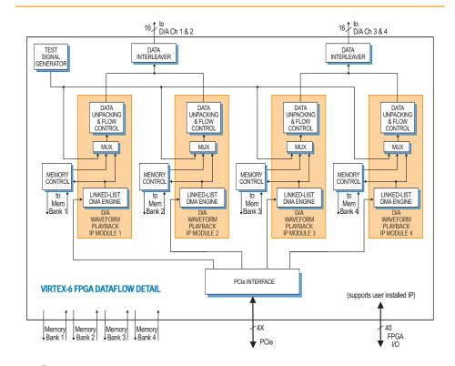
D/A Waveform Playback IP Module
