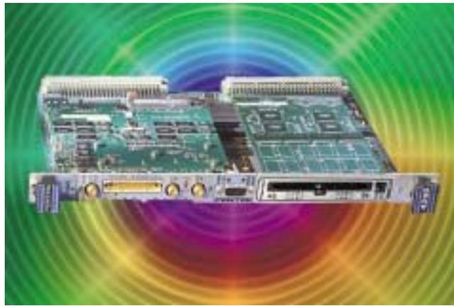
*Model 4295 - four MPC7410 PowerPC processors on a single-slot 6U VME board*
