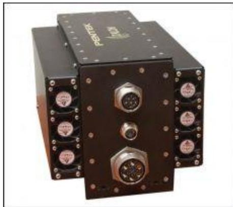
Conduction cooled SFF recorder subsystem with A/D converters, digital down converters, and removable 15-TB SSD storage supports recording rates up to 4 GB/sec. Removable air cooling jackets are installed on each side for lab operation.
