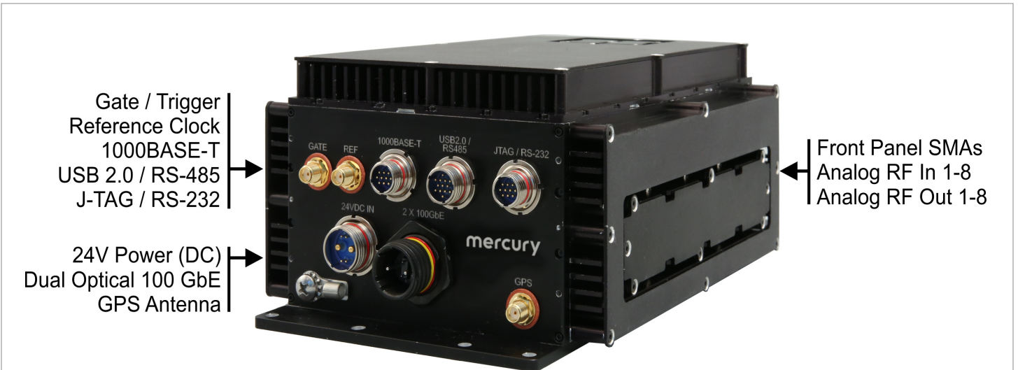
Figure 1. Example of RFSoc-base SFF ruggedized sub-system. The Quartz Model 6353 provides 8 channels of remote data acquisition and generation, local ARM processor system controller, FPGA fabric for DSP, and dual 100 GbE optical interfaces with VITA-49 data protocol.
