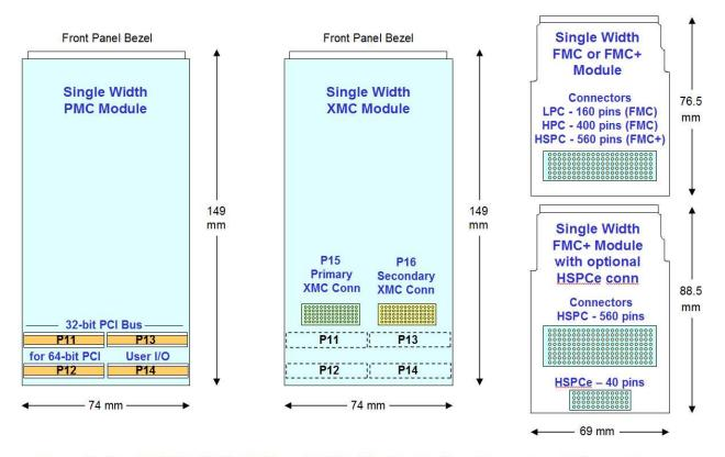
Figure 1. Single PMC, XMC, FMC and FMC+ Module Outline Dimensions & Connectors (drawn to scale, for comparison)
