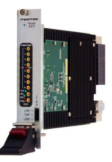
Figure 5. Pentek FlexorSet Model 5973-316 8 Ch A/D 3U VPX Module based on 5973 3U VPX Virtex-7 FMC Carrier and 3316 FMC module
