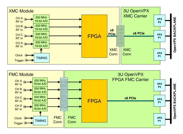
Figure 3. Simplified block diagrams comparing XMC and FMC 4-Channel A/D Software Radio Modules for 3U OpenVPX
