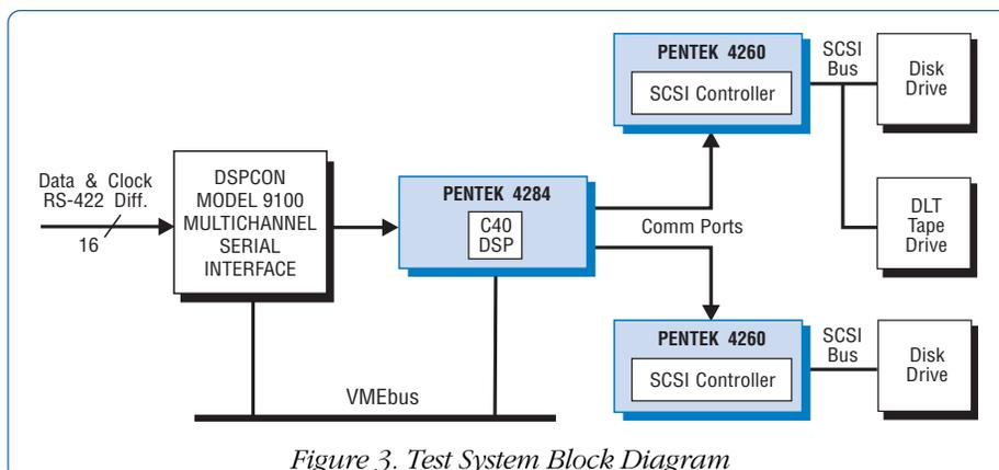
Figure 3. Test System Block Diagram
