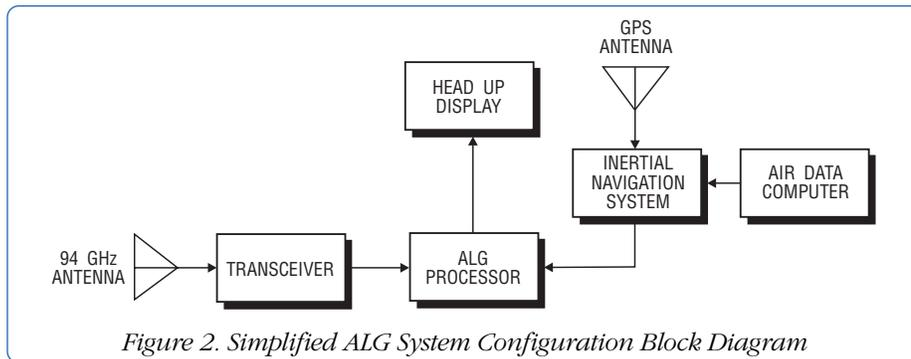
Figure 2. Simplified ALG System Configuration Block Diagram
