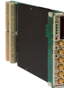
Model 7158 Software Radio XMC for Very Wideband Signals
