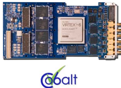
Model 71620 Software Radio XMC with Virtex-6 FPGA
