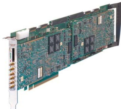
Model 7751D 512-Channel Software Radio PCI Express Board
