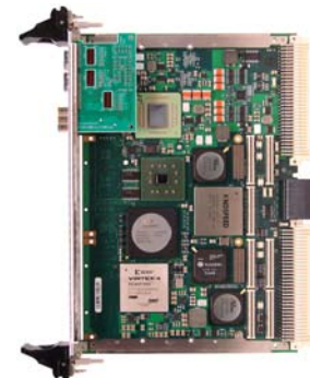
Model 4207 VME/VXS Processor with two PMC/XMC Sites
