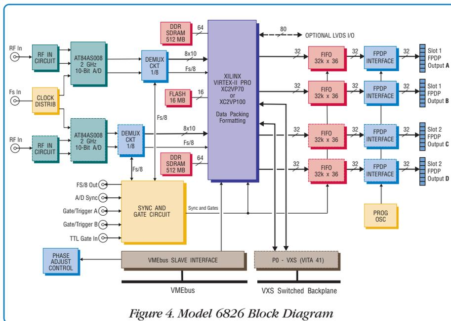
Figure 4. Model 6826 Block Diagram
