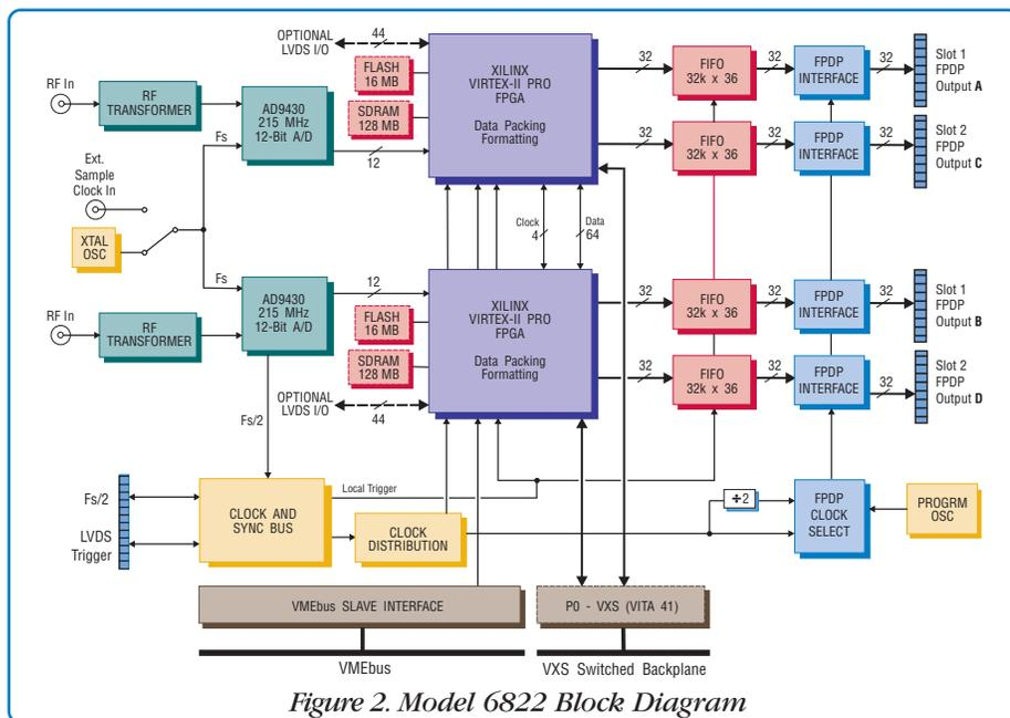
Figure 2. Model 6822 Block Diagram
