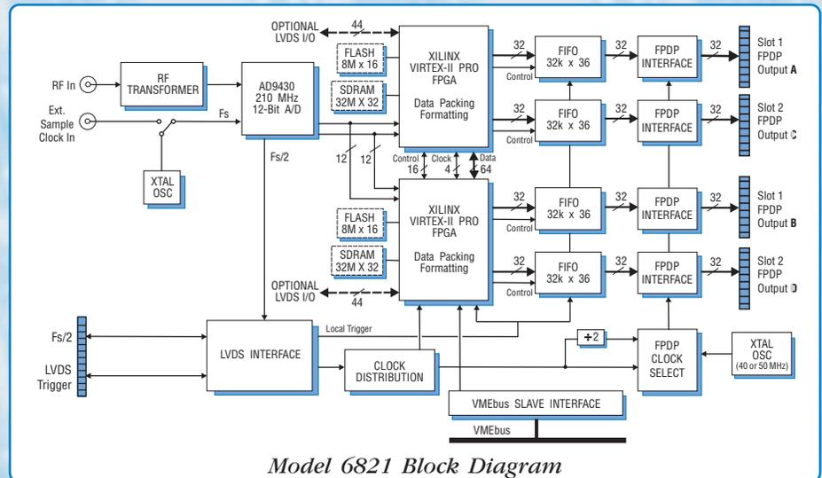
320 MB/sec. One port per FPGA is attached to the 6821 front panel, while the second is available on an optional second-slot panel. A data demultiplexing mode splits the data stream between each pair of FPDP ports reducing data rates by a factor of up to eight to support
