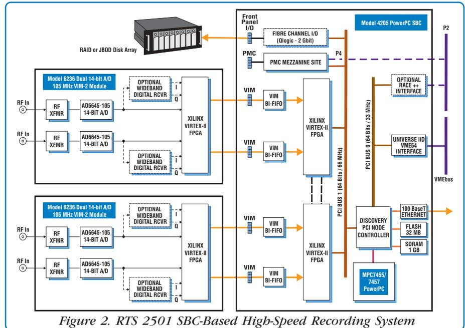
Figure 2. RTS 2501 SBC-Based High-Speed Recording System
