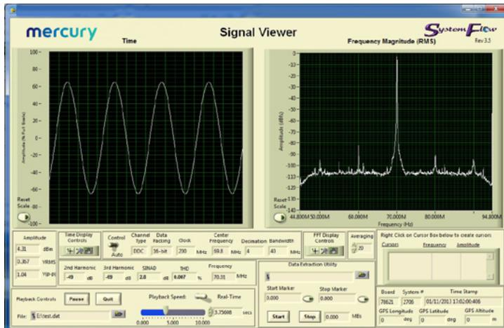
The SystemFlow Signal Viewer includes a virtual oscilloscope and a virtual spectrum analyzer for signal monitoring in both the time and frequency domains. You can download and install the free SystemFlow Simulator to your desktop or laptop PC.
